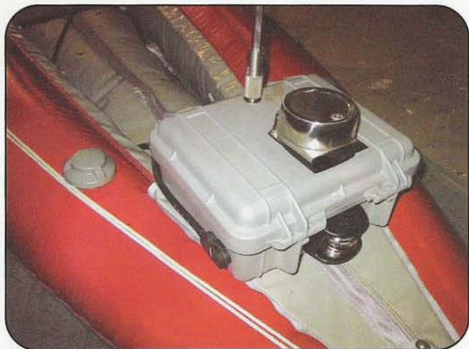
Photo D. The Pelican box at the stern carries the white LED navlight seen in photo C, as well as a bayonet-mount J-pole antenna and yacht horn. Note waterproof connector.
