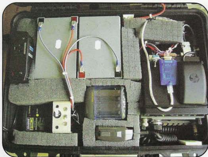
Photo B. The inside of the black Pelican case at the bow. Contents include a KPC-3+ packet TNC, Yaesu 290, USB-serial interface for Mac laptop, Garmin GPS-35, 24 amp-hours of 12-volt sealed lead-acid batteries, Micro-M+ solar charger, AC unit, Statpower inverter, Maha Ni-MH charger, bicolor navlight retrofitted with Luxeon 1-watt LED emitters, 350-mA constant-current source for same, and Mobri radar reflector.
