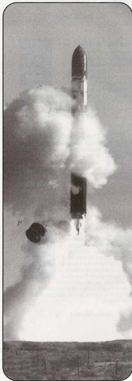
The main engines of a Dnepr LV fire just as it clears the launch silo. The large, dark cylinder is the gas-generator that ejects the Dnepr from the silo prior to engine start; this is known as “cold launch,” which allows the silo to be reused. (Photo courtesy of Richard Hambly, W2GPS)
