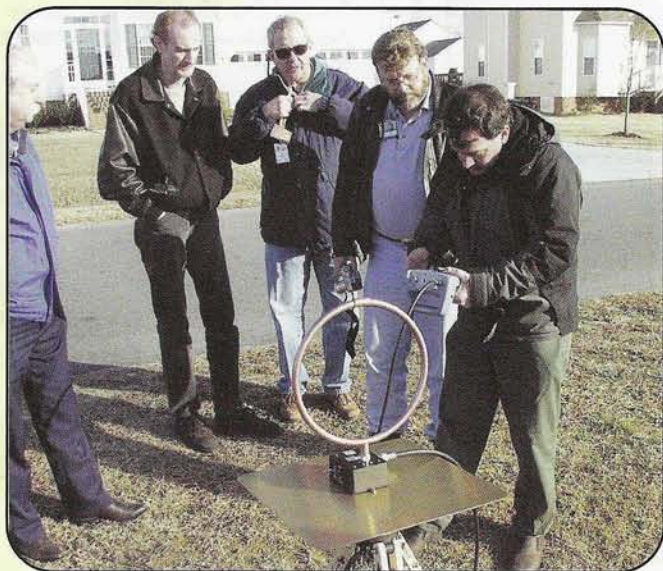
Bill Godwin; Will Roberts, AA4NC; Tom Brown, N4TAB; Frank Lynch, W4FAL; and Amperion's Garrett Durling measure BPL signal levels from the ground-mounted pedestal.
