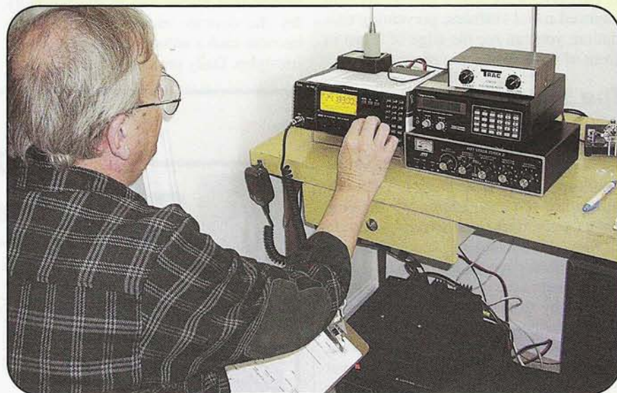
Tom Brown, N4TAB, listens on 24 MHz at Roland Erickson, WA0AFW's home near the second trial area. The signal was weak, but audible on Roland's attic-mounted dipole, about a half mile from the BPL site.
