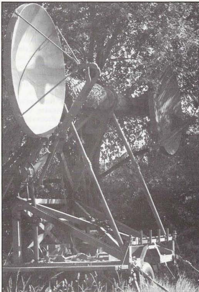
Dual diversity antenna system used in troposcatter propagation by the US Army. (Courtesy of US Army)
